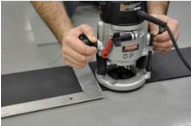
Make a relief by cutting 1/8" deep relief on back
